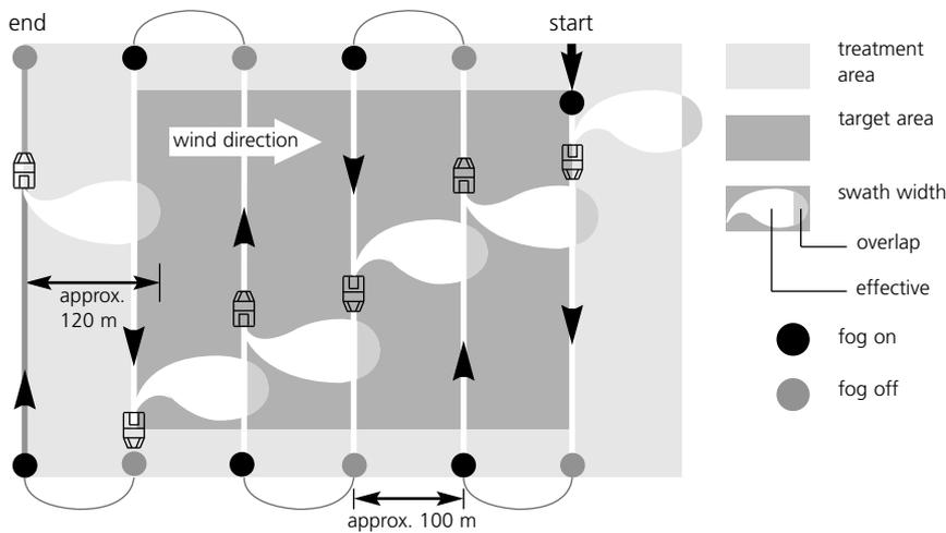
Example of a large area treatment using the Fontan Mobilstar, taking into account wind direction and swath width.
