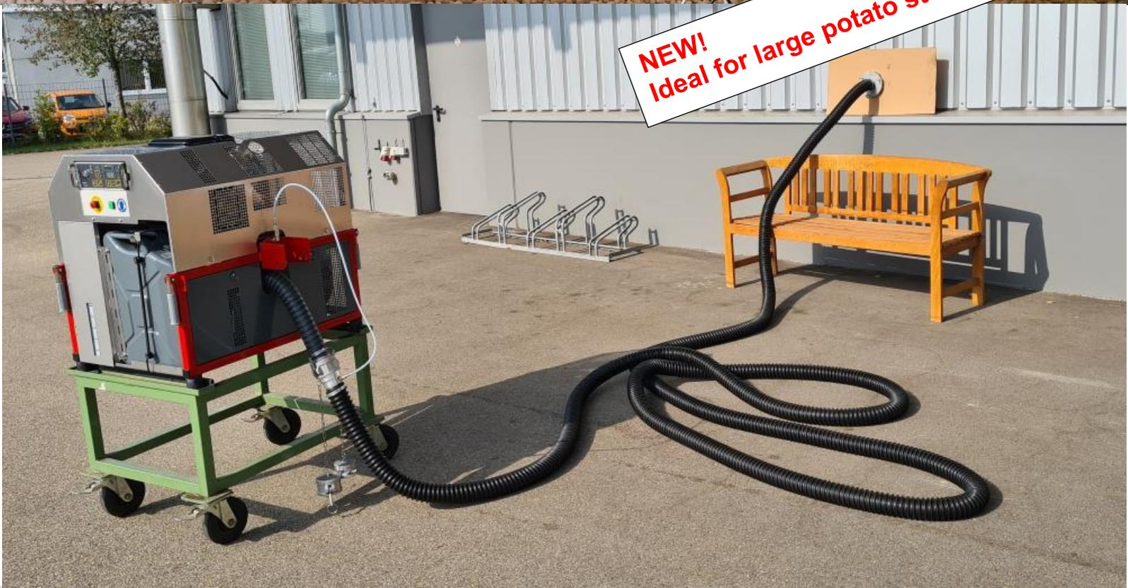
The fontan® Mobilstar EK was specially developed for the application of modern germ inhibitors such as ARGOS. It does not generate an open flame and the ignition temperature is never reached. Due to the high output rates of 5 - 100l / hour, even large warehouses can be treated efficiently in a short time. The device works independently and generates ideal droplet sizes for use in potato sprout inhibition.
